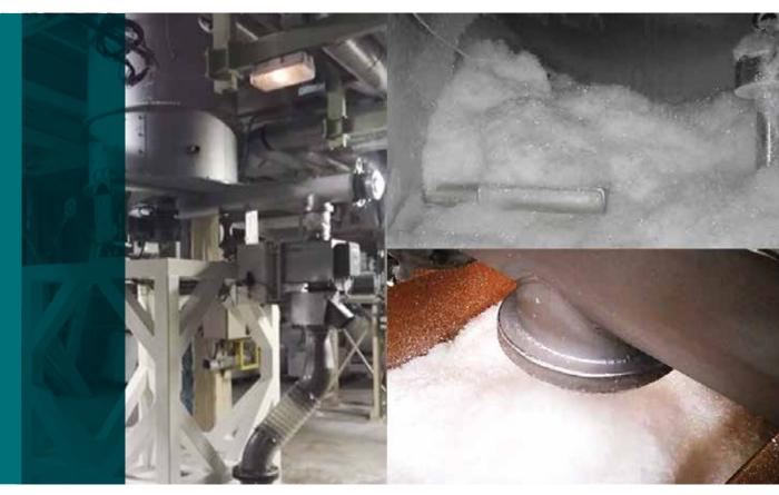
By utilizing the Simplex feeder difficult to feed materials such as PET flakes, glass fibers, and regrind.
