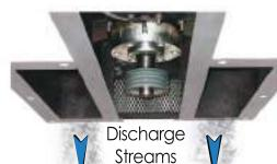
Automatic recirculating lubrication & temperature control system extends bearing cartridge Life Fully lined open rotor improves first pass yields
